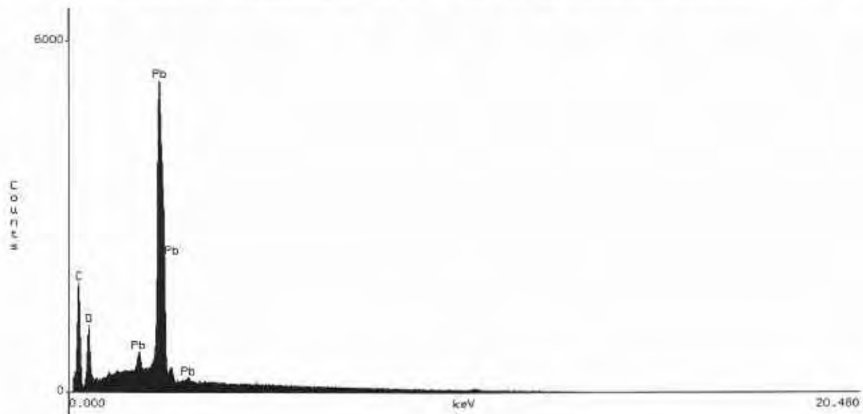
Figure 4-16 SEM image (top) and EDS spectra (bottom) of Pb-carbonate corrosion products formed on partially submerged coupon L294. Sources: image file L294_2.BMP and spectra file L294_1.doc located on disk in "WIPP-FePb-3 Supplemental Binder D".
